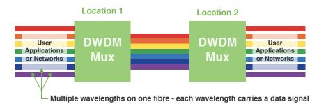
DWDM continues to evolve over time. Some DWDM implementations are set up to allow for 96 wave lengths of 200Gbps per wavelength or 48 wavelengths of 400Gbps per wavelength.
